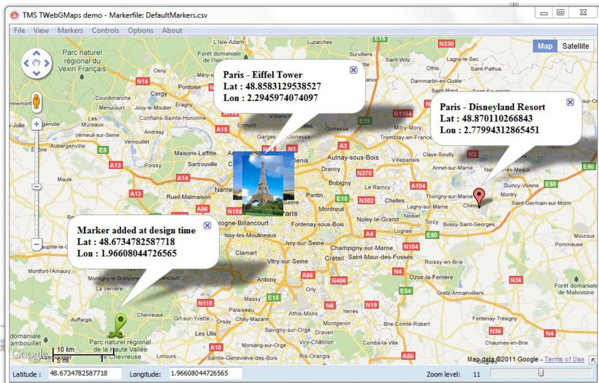
On the left hand side, a PNG image is used as marker. In the middle section, two JPEG images are displayed as marker. On the right hand side, a standard Google Maps balloon marker is used, as the marker was created with an empty icon property.
