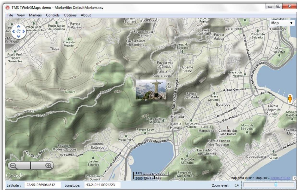
The position of the Google Controls has been changed : PanControl to the TopLeft position, MapTypeControl to TopRight. The ControlsStyle is changed to Android style. Note the zoom control in the bottom left corner displayed in Android style.
