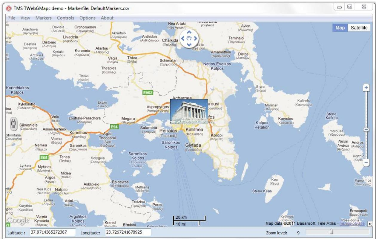
In this sample, the position of the Google Controls has been changed : PanControl to the TopCenter position, ZoomControl to RightCenter, ScaleContol to BottomCenter and StreetviewControl to LeftCenter.
