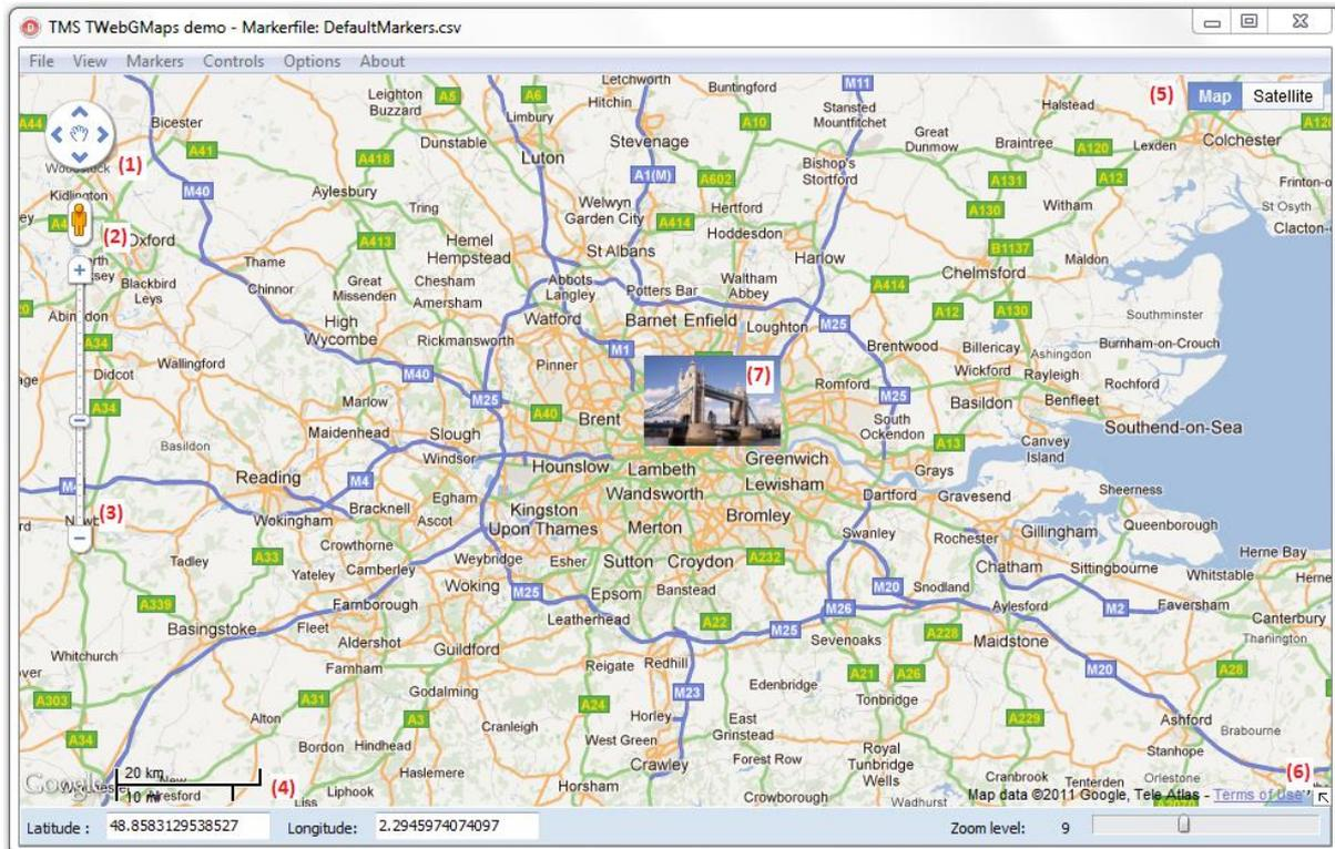
The core part of the TMS WebGMaps is the TWebGMaps control, a VCL component integrating the Internet Explorer browser and exposing properties, methods and events to control Google Maps. Additional Google Maps controls can be optionally enabled on the map, i.e. a PanControl (1), a StreetViewControl (2), a ZoomControl (3), a ScaleControl (4), a MapTypeControl (5) and an OverviewmapControl (6).
